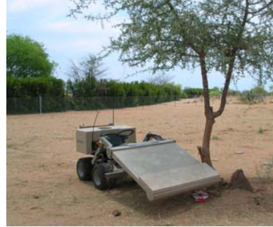
NIITEK Minestalker™ Detects anti-tank landmines, explosives, and buried anomalies through remote subsurface visualization.
