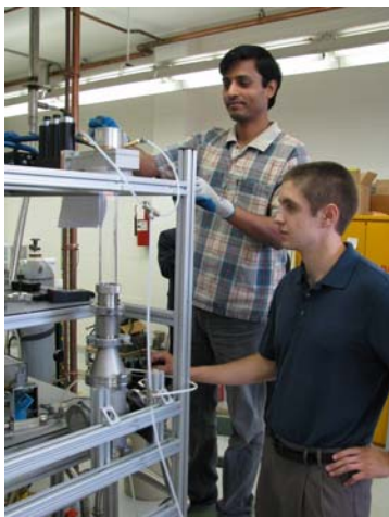
Graduate students Vivekanand Kumar (left) and Boris Chernomordik (right) demonstrate the UofL patented, atmospheric plasma jet reactor that can make kilogram quantities of nanowires out of a variety of metal oxide materials.
