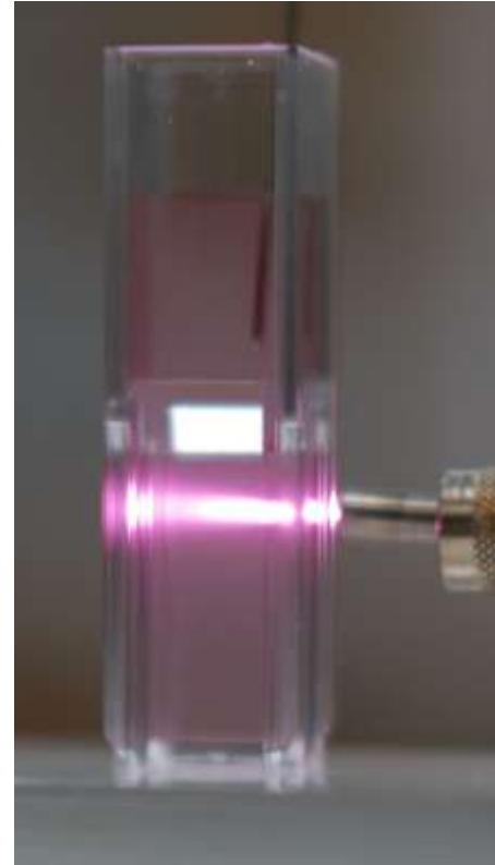
Gold/Silica + Laser Visibly higher scattering of laser light
