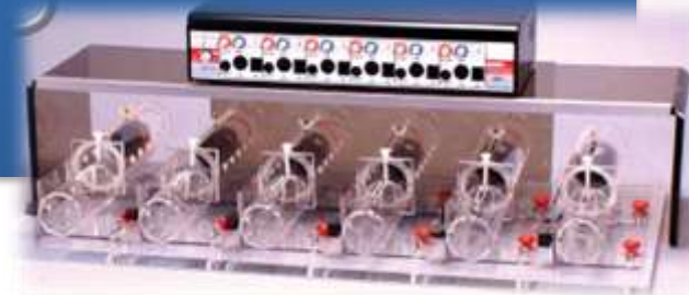
CODA 6 device measures blood pressure non-invasively by tail-cuff using sensitive pressure volume recording sensors
